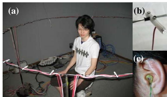
Fig. 1: Reciprocal system for HRTF measurement (a) Overview of system, (b) Close up of microphone, and (c) earplug speaker.
