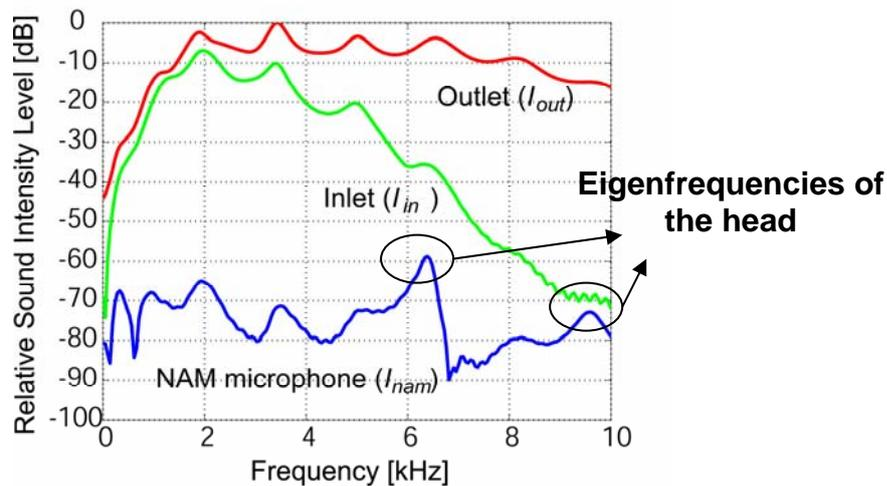
Fig. 3 – Sound intensity level at outlet and inlet of vocal tract, and NAM microphone
