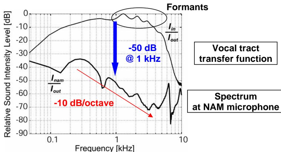
Fig. 4 – Attenuation characteristics at NAM microphone
