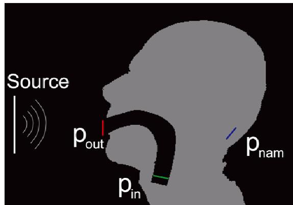
Fig.2 – Simulated region including the head, vibrating plate, and receivers
