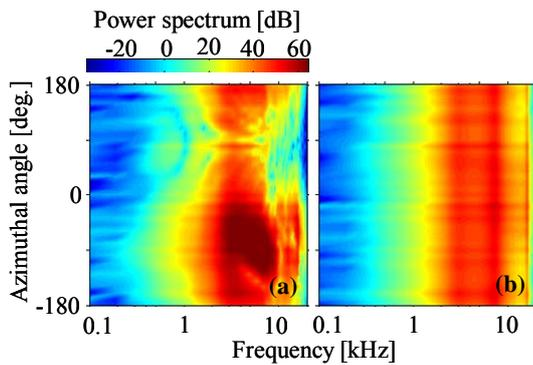
**Figure 7:** Near-field transfer function contour patterns of (a)  $H_{Ear}$  and (b)  $H_{Center}$  measured with ED-29689.
