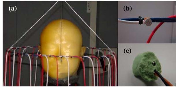
**Figure 1:** Reciprocal system for HRTF measurement (a) Overview of system, (b) Close up of microphone, and (c) earplug speaker.
