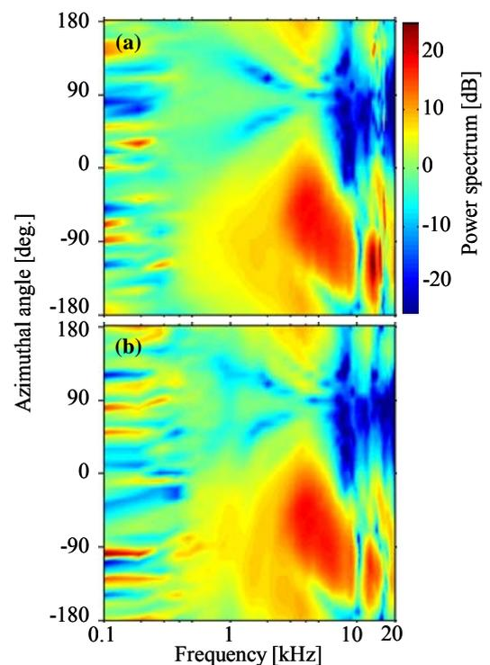
**Figure 6:** Far-field (1-m distance) HRTF contour patterns of left ear of dummy-head. (a) Using DTEC-30008 and (b) using ED-29689.
