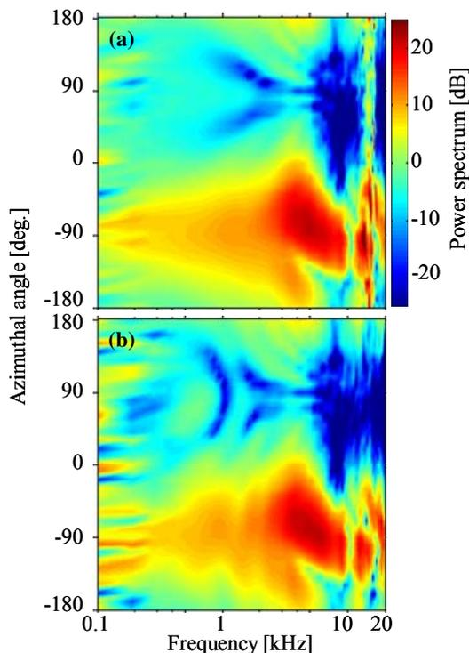
**Figure 5:** Near-field (0.2-m distance) HRTF contour patterns of left ear of dummy-head. (a) Using DTEC-30008 and (b) using ED-29689.
