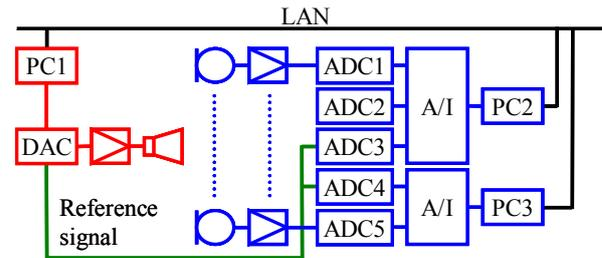
**Figure 2:** Block diagram of electroacoustic equipment.
