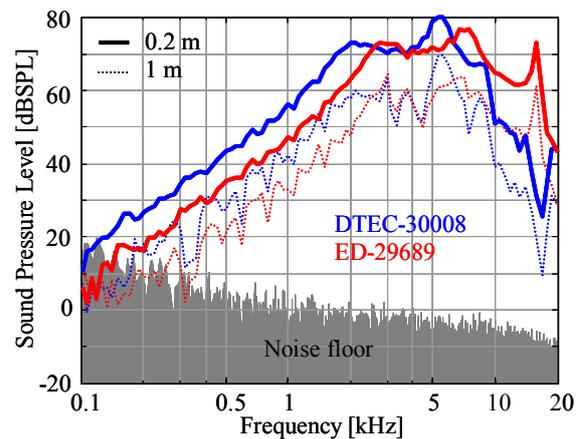
**Figure 3:** Frequency responses of earplug speaker in near-field.
