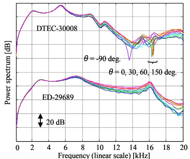
**Figure 4:** 12-direction (30-degrees apart) frequency responses of two miniature speakers in horizontal plane.
