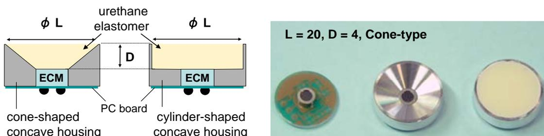
Figure 1: Structures and photographs of body-conducted sound sensor.
