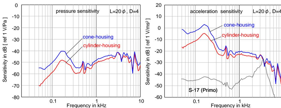
Figure 2: Pressure and acceleration sensitivity of body-conducted sound sensors.
