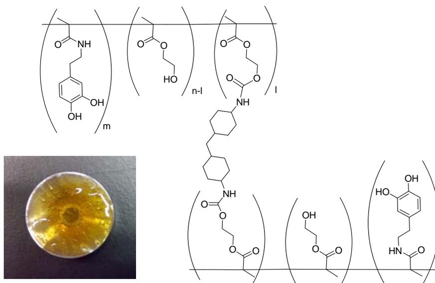
Figure 4: Proposed structure of gel obtained by crosslinking reaction and poly(DMA-co-HEMA)-crosslinked gel-deposited body-conducted sound sensor.
