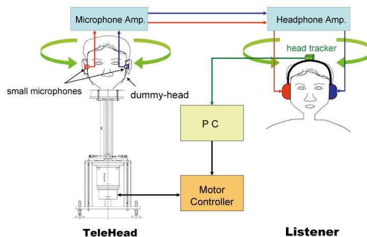
Figure 1 – Schematics of *TeleHead*, which is rotatable dummy head that quietly tracks listener's head movement in real time.
