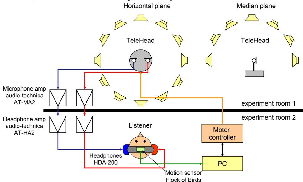
Figure 5 – Schematic of the sound localization experimental system. When a listener localizes stimuli through binaural signals, the *TeleHead* is placed at center of the speaker array and the binaural signals provided using either the stereo microphones, simple dummy head or personal dummy head are presented to the listener sitting in another room via headphones.
