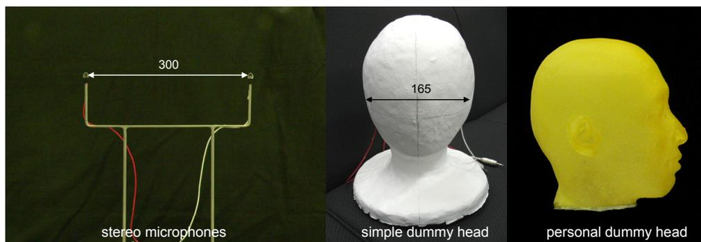
Figure 2 – Photographs of stereo microphones, simple dummy head, and personal dummy head used in experiment.
