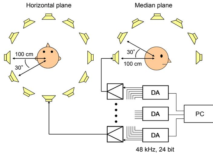
Figure 4 – Schematic of the sound localization experimental system. When a listener localizes stimuli with his ears, he sits at center of the speaker array.
