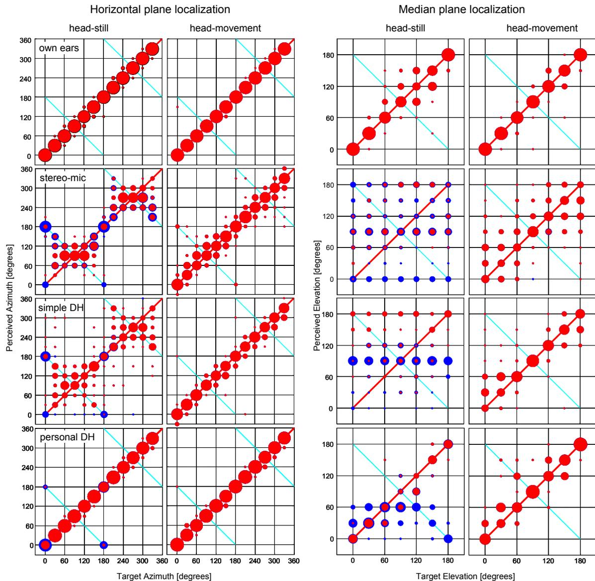
Figure 6 – Pooled horizontal and median plane sound localization results with listeners’ own ears, stereo microphones, a simple dummy head, and personal dummy heads in head-still and head-movement conditions. Blue circles represent in-head localizations and red circles represent out-of-head localizations. Area of each circle is proportional to localization rate.
