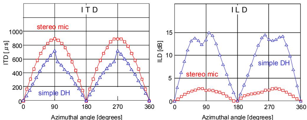
Figure 3 – ITD and ILD variations of stereo microphones (red) and simple dummy head (blue) with azimuthal angles.
