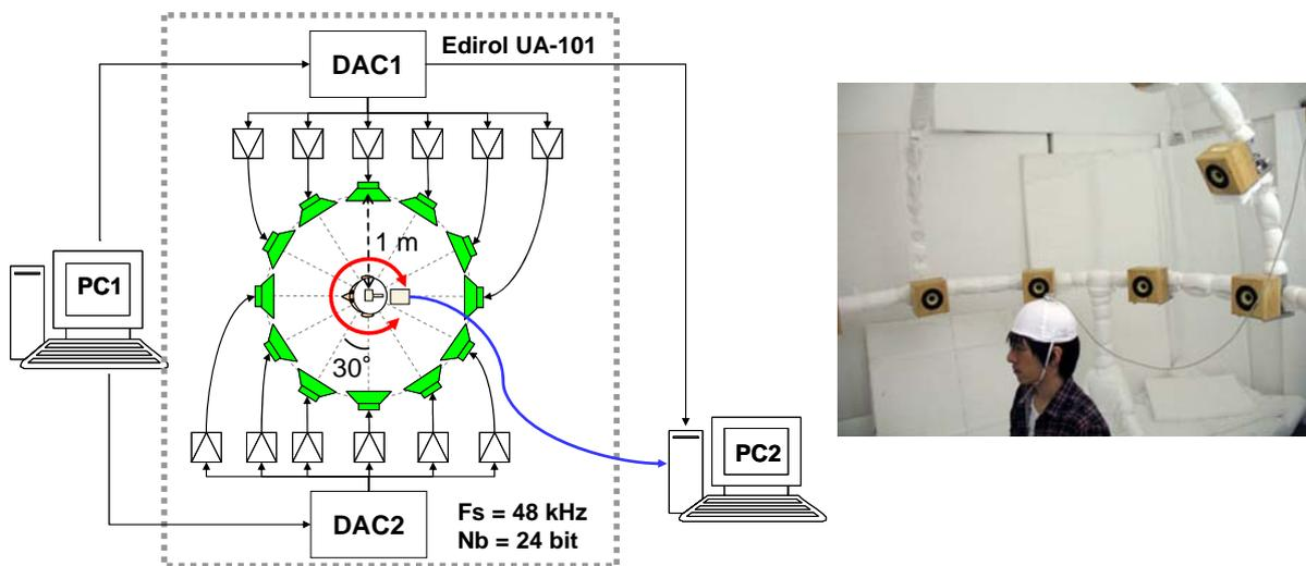
Figure 1 – Block diagram of experimental system (left) and photograph of experiment room (right). PC1 was used to for stimuli presentation for sound localization experiment. PC2 was used to simultaneously record sound stimuli and subject's head movement data.
