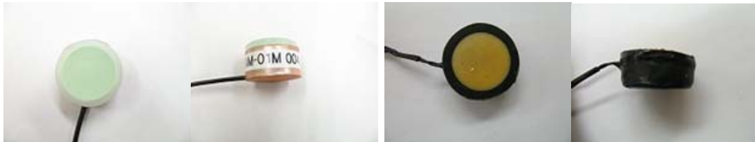
Fig. 3. A soft-silicon type (left) and a urethane-elastomer type (right) NAM microphones.
